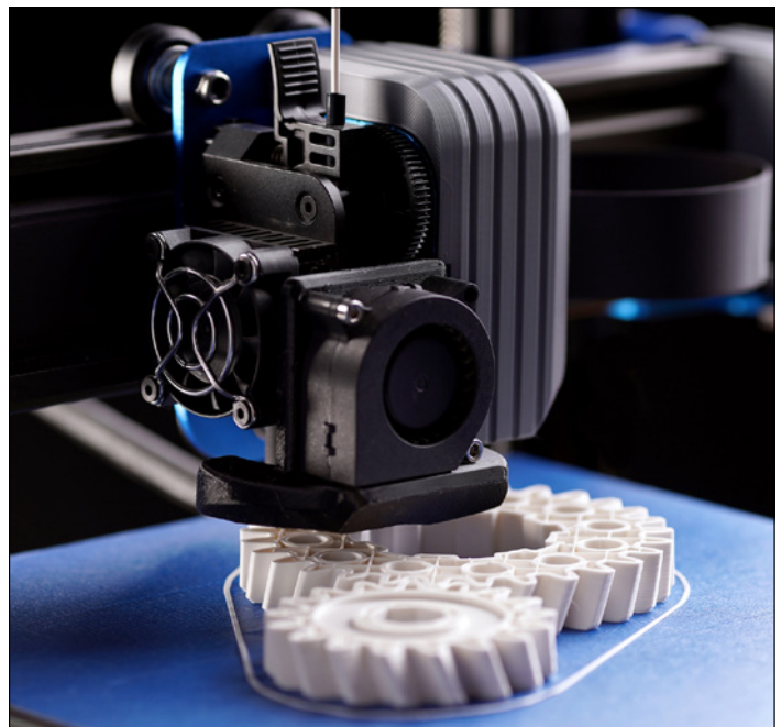
Figure 5. FDA recently released a guidance document on technical considerations for additive-manufactured medical devices. 13 Here, the gantry with x-carriage and printhead of a fused deposition modeling (FDM) 3D printer producing white helical gears. Image courtesy Dreamstime (ID 241350887) © Roman Boettcher.
