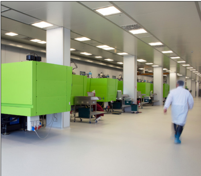
Figure 4. Cleanroom molding of biomedical products—a common setting among medical product manufacturers. Image courtesy Dreamstime (ID 48273907) © Moreno Soppelsa.
