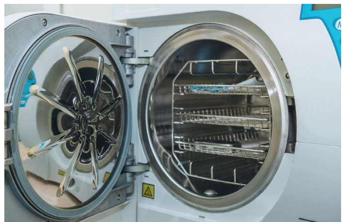
Figure 6. Device manufacturers are responsible for validating their products to the cleaning, disinfection, and sterilization methods dictated by their bill of materials. Here, a steam autoclave. Image courtesy Dreamstime (ID 169613542) © Yuri Tabolin.
